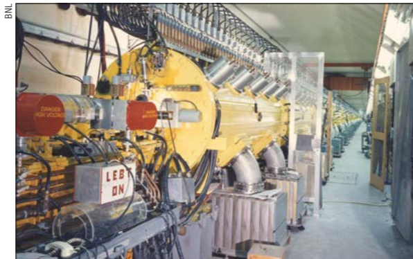
Brookhaven's linear accelerator is 144.8 m long and feeds a beam either to the BLIP or the Booster accelerator.
